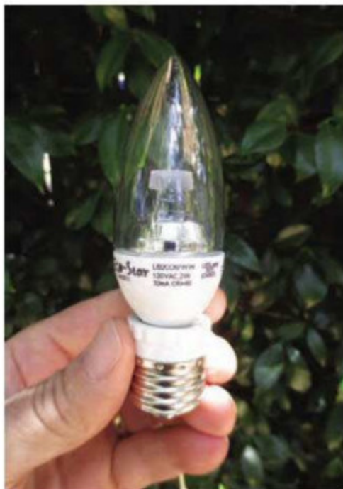
A 2-watt LED is bright, but the bulb needs a reflector.
